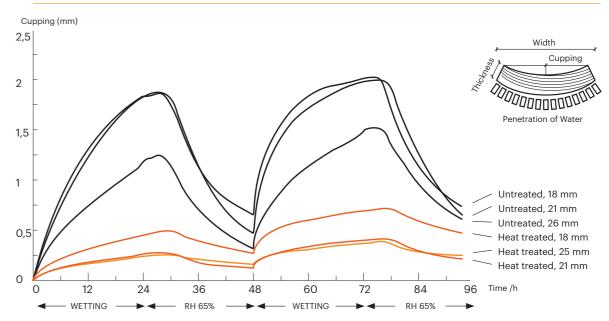
Cupping of exterior cladding boards: Comparison between LunaThermo-D and untreated Scandinavian pine and spruce in different thicknesses.
